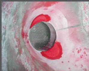
PUCEST® Tix was developed especially for the repair of PUCEST® wear protection systems.
