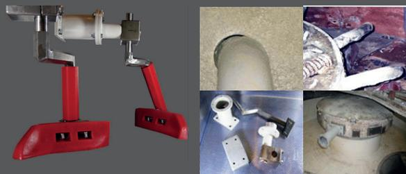
Torsion spring-loaded mixing arm for the retooling of pan mixers
