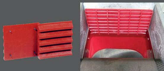
Deflectors for transfer points with pocket buffer, for a grain size from 0 to 32 mm or with step profile, for a grain size from 0 to 75 mm, depending on the profile of requirements.
