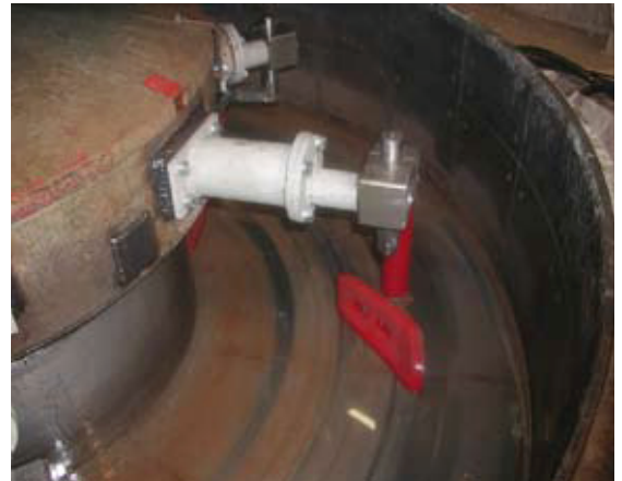
Fig. 2 Converted mixer with Pucest console arm and mixing blade.
