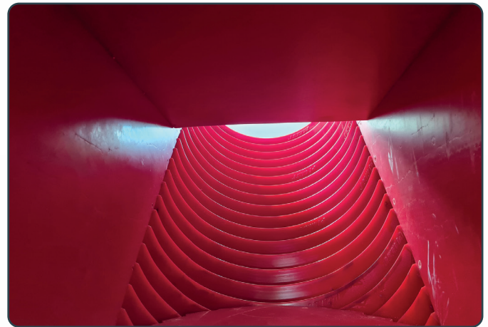
SZ panels as a lining in an outlet hopper in conjunction with PUCEST panels.
